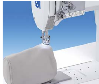
868-390322 CLASSIC Topstitching operations with left-handed post bed in narrow radii in the production of headrests
