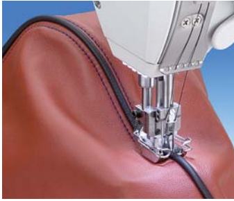
868-290322 CLASSIC Effective seam appearance and constant seam margins when sewing decorative welt seams
