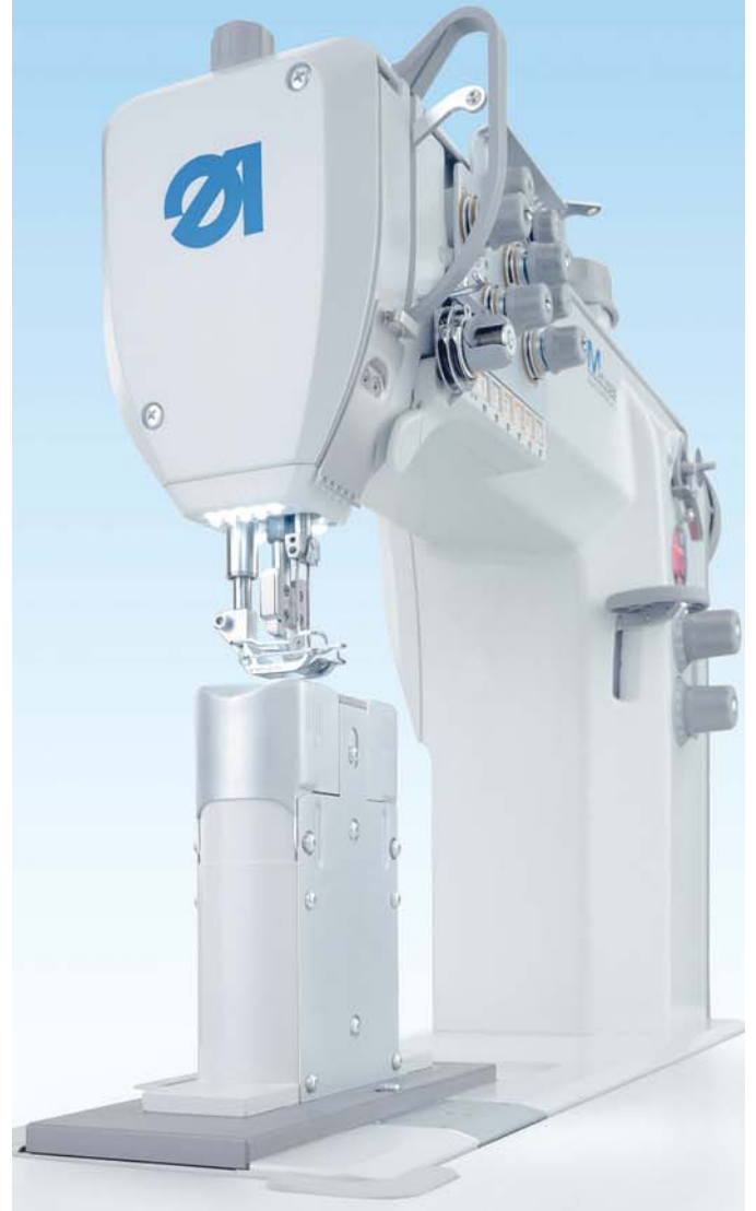
868-390322 CLASSIC Topstitching operations with left-handed post bed in narrow radii in the production of headrests
