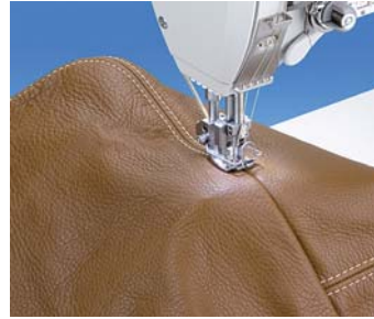
868-290322 CLASSIC Tight stitch formation and constant seam margins when topstitching furniture leather by means of sewing equipment with compensating foot and presser foot with integrated seam center guide
