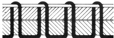
Illus. c: Needle thread tension too high or Underthread tension too low
