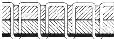
Illus. b: Needle thread tension too low or Underthread tension too high
