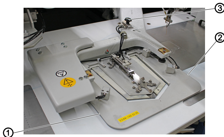
Fig. 31: Removing the transfer plate
