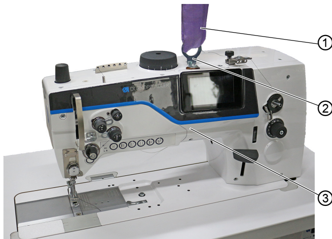
Fig. 51: Inserting the machine head (1)
