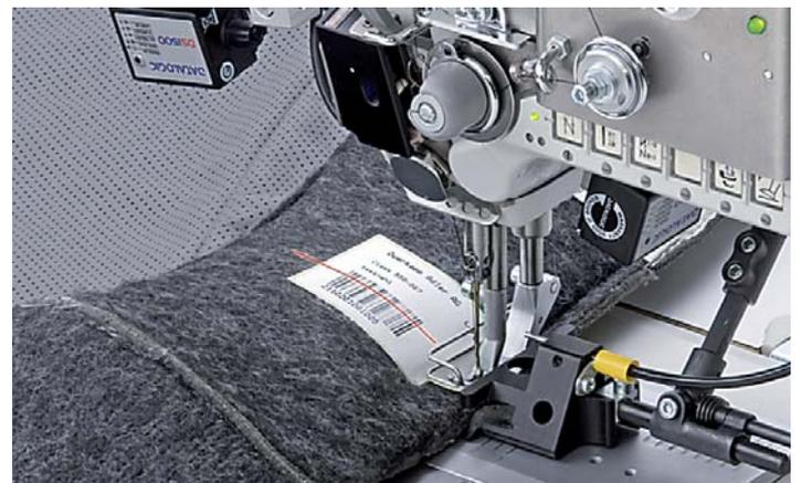
Class 550-867 – Identification of Endlabel-Barcode with all relevant information of the complete sewing process
