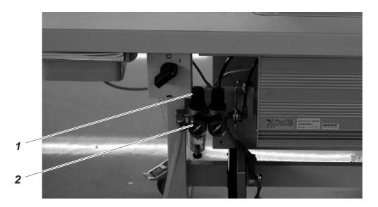
The pneumatic system of the machine and its auxiliary equipment must be supplied with compressed air containing absolutely no water or oil.
