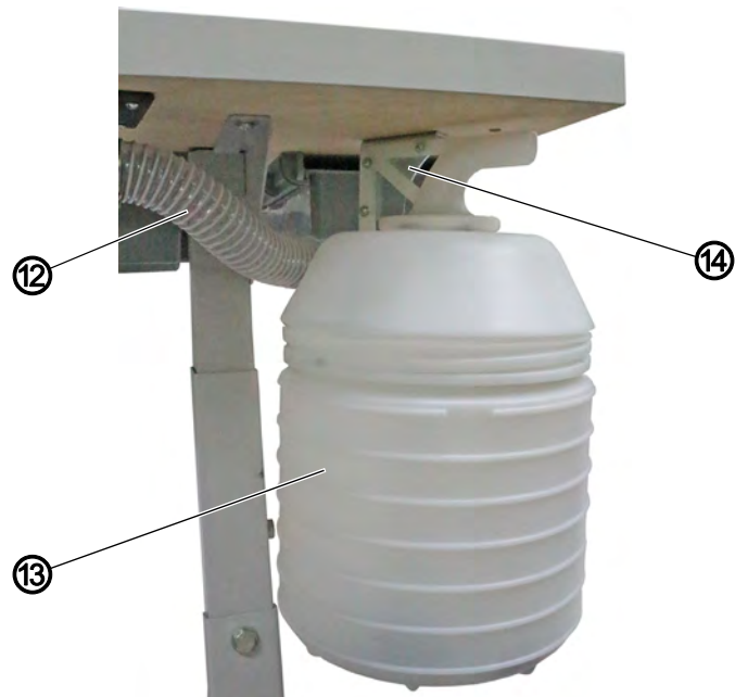
Fig. 5: Assembling the extraction system (5)
