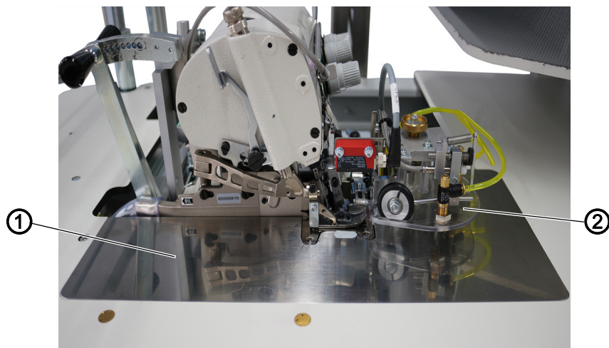
Fig. 4: Disassembling and assembling the fabric sliding plate (1)
