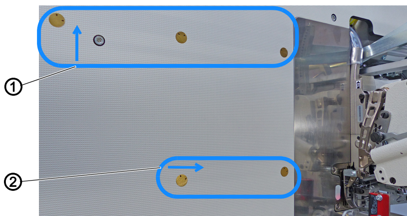
Fig. 23: Adjusting the air nozzles in the tabletop (1)
