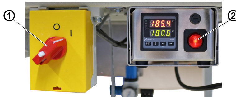
Fig. 23: Switching on the fusing station
