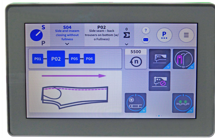
Fig. 69: Commander Pro control panel
