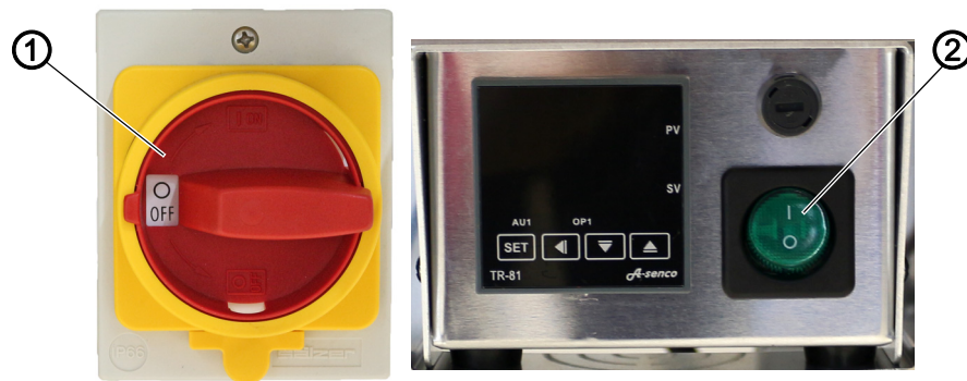
Fig. 8: Switching on the fusing station
