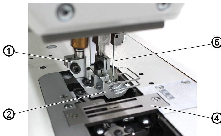
Fig. 1: Disassembling the sewing equipment
