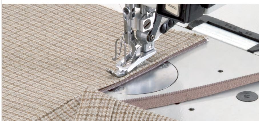
**275-140342-01 E2 – Runstitching and topstitching of wing pocket openings** with swivable edge guide;
