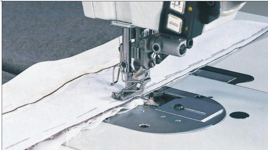
**275-740642-01 E104 (8 mm) – Attach waistband and simultaneously cutting the edge**
