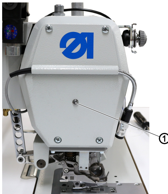
Fig. 57: Setting the height of the locked sewing feet (1)
