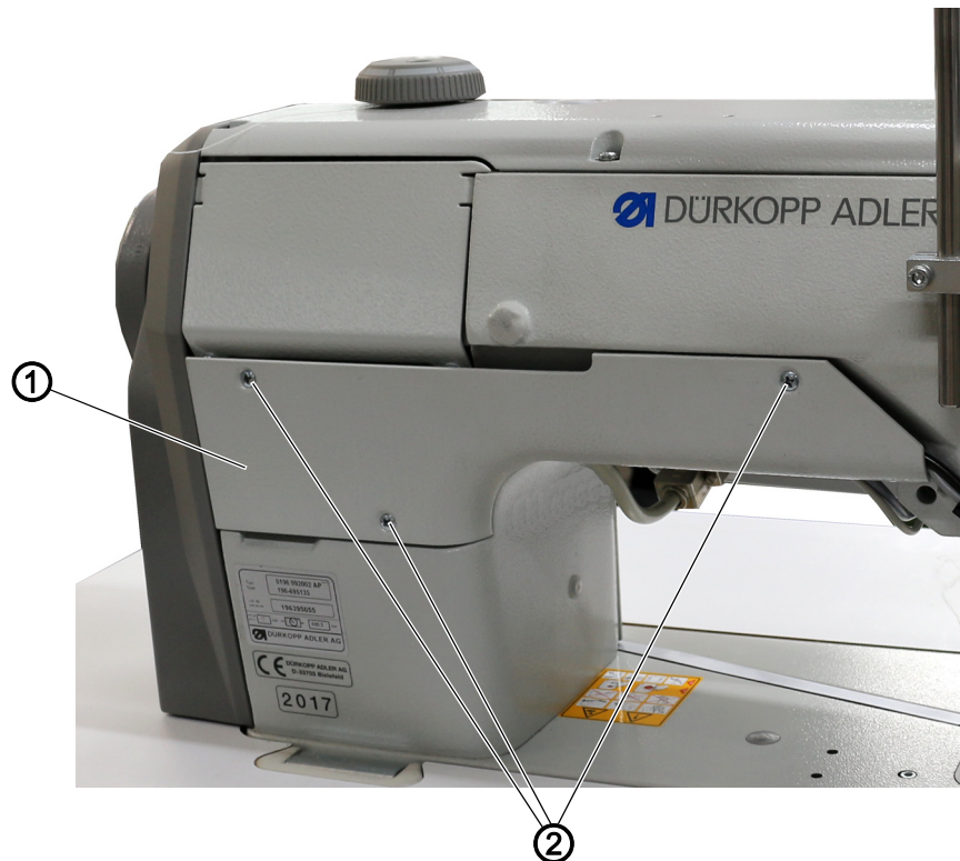
Fig. 9: Disassembling and assembling the rear cover
