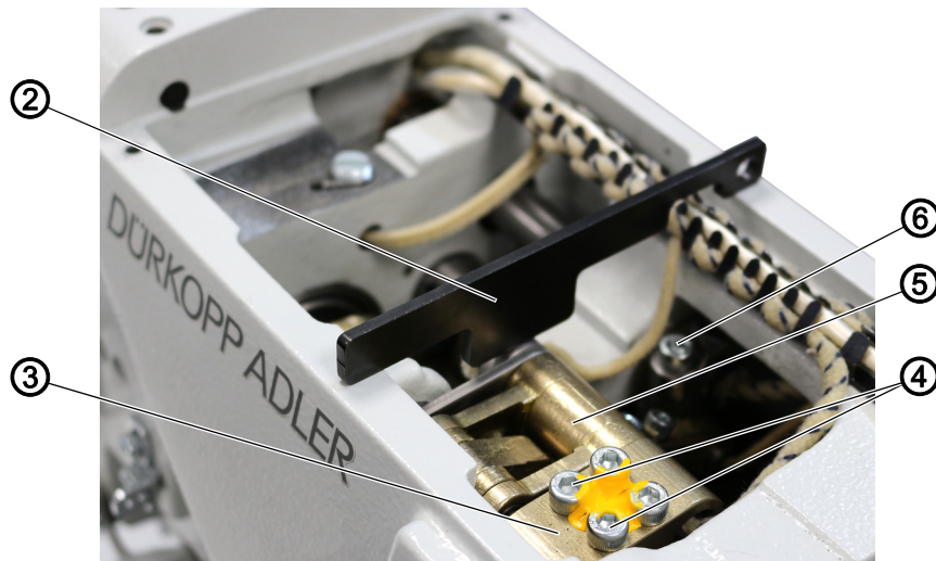
Fig. 50: Setting the stroke adjusting range and the timing of the walking foot stroke movement (2)
