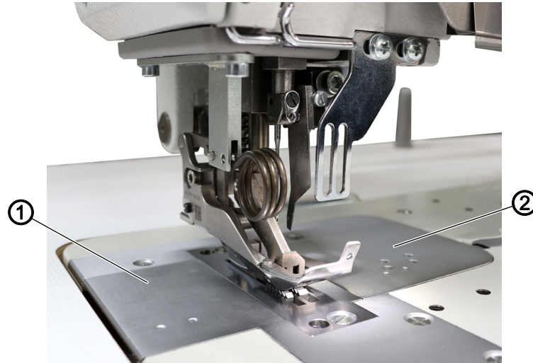
Fig. 16: Opening and closing the hook covers (1)
