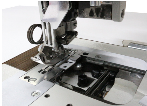
Fig. 18: Opening and closing the hook covers (3)
