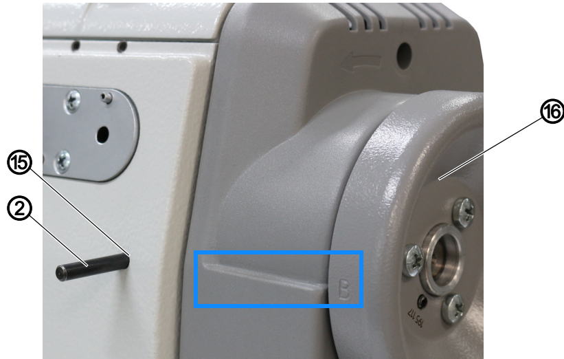
Fig. 25: Setting the adjusting disk relative to the arm shaft crank (5)
