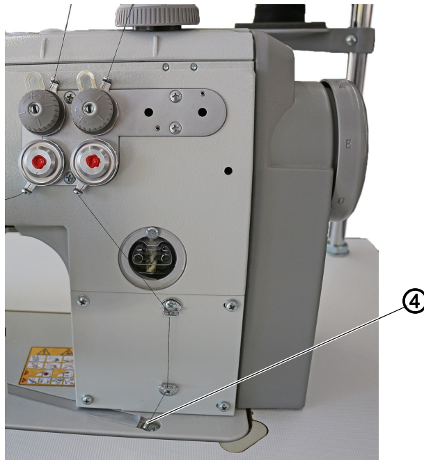
Fig. 77: Calibrating the electronic hook thread tensioner (2)
