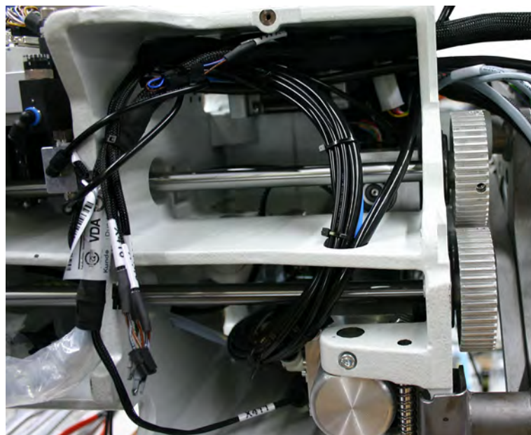
Fig. 5: Routing compressed air lines (3)
