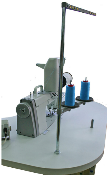
Fig. 56: Assembling the thread reel holder (final state)
