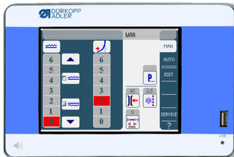
Fig. 42: Control panel OP7000
