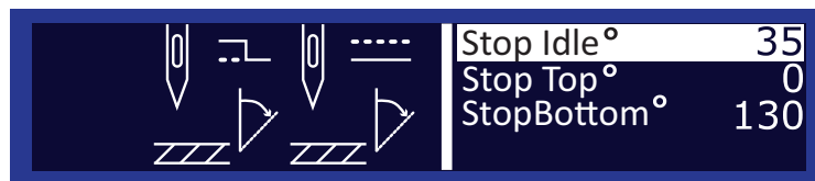
Fig. 50: Sub-item Stop Positions
