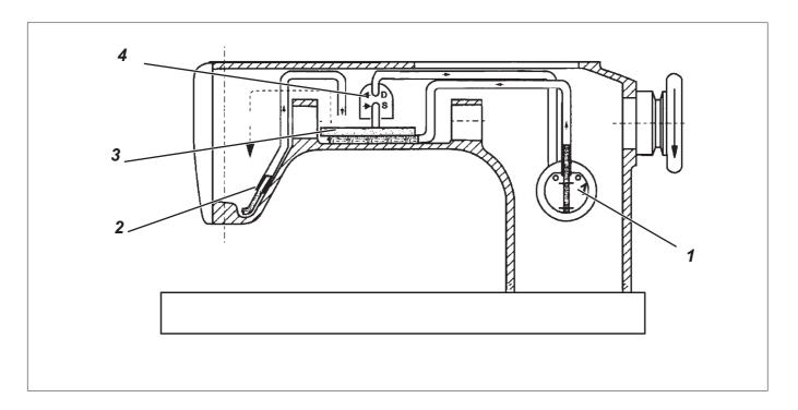
The oil runs from the oil tank 1 to the oil sump 3. From there, the lubricating points in the arm and head sections are provided with oil.
