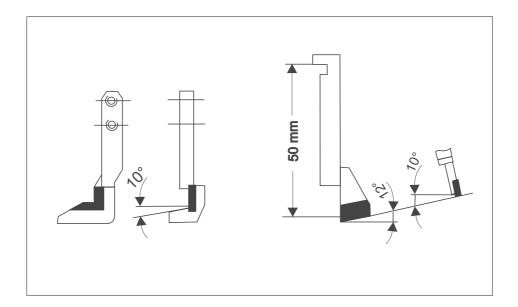
Resharpen the blades that are made in hard metal (Widia) diamond disc.
