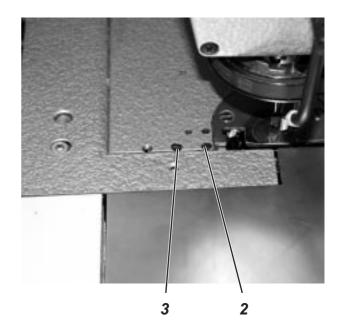
To replace and adjust the blades, dismantle the tread scissors.
