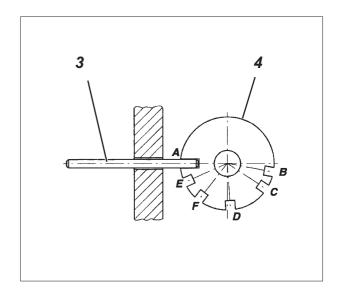
By means of the retention pin 3 and the adjusting disc 4 integrated in the toothed belt wheel, the sewing machine can be locked in the current setting positions.
