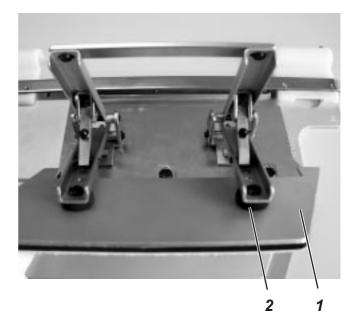
Secure clamping plate 1 with pressure piece 2 and circlip 3 at the tension levers.
