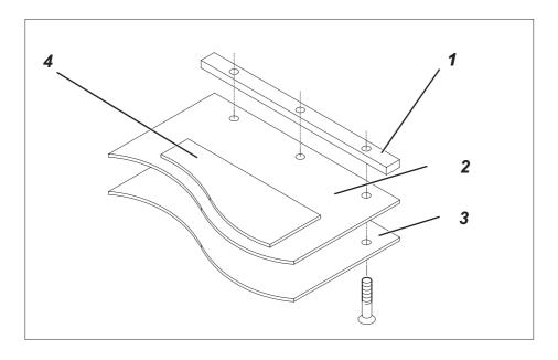
Connect bed-plate 3, intermediate sheet 2 and threaded shackle 1 with three countersunk screws.
