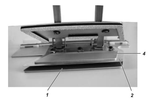
Adhere emery cloth onto the top surface of the bed-plate 1 in the area of the sewing material.
