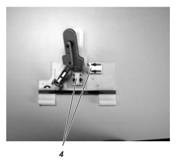
Secure material stops 4 with hexagon nuts 6 and screws 5 to the bed-plate.
