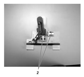
Material clamps for flaps can be equipped with up to 4 material stops 1, while clamps for waistband extensions can have max. two stops 2.
