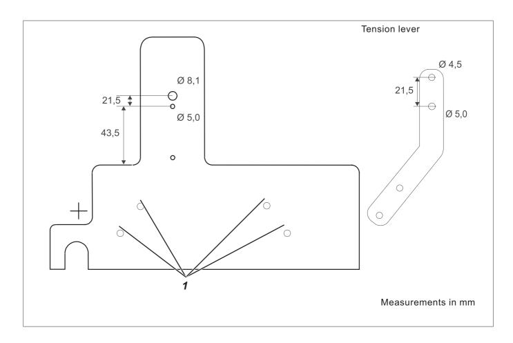
The bed-plate and the clamping plate are already equipped with holes for the clamping element. Depending on the handling, the clamping element can be positioned to the right or the left respectively.
