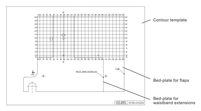
Upon the setting up of the sewing programme, the exact seam contour must be entered in the Dacs739 software. Therefore, the individual coordinate points of the seam contour must be determined
