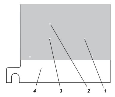
Place bed-plate 4, intermediate sheet, clamping plate and pointing plate on top of each other and secure with two countersunk screws, washers and nuts.
