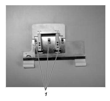
To be able to adjust the material stops 1, the intermediate sheet must be equipped with slots.
