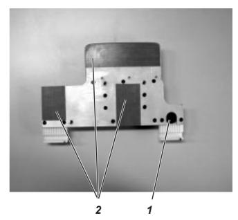
To ensure that the material clamp can be moved with minimum friction across the table-top, a sliding foil must be adhered to the base of the clamp.
