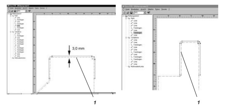
After the sewing programme has been set up by means of the Dacs739 software, contour 1 of the material clamp can be stitched to provide a template.
