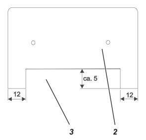
For the installation of the stops 1 on a material clamp for flaps, the clamping plate 2 has to be unlocked at the base 3.
