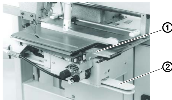
Fig. 15: Setting the working range, angle and length
