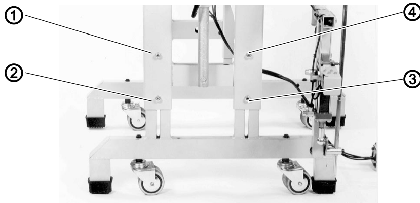
Fig. 31: Setting the working height
