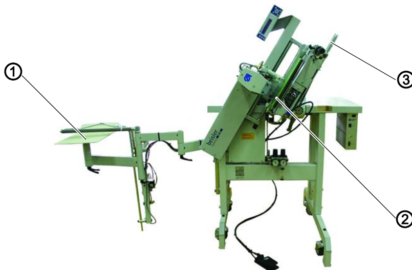
Abb. 23: Swiveling up the machine head
