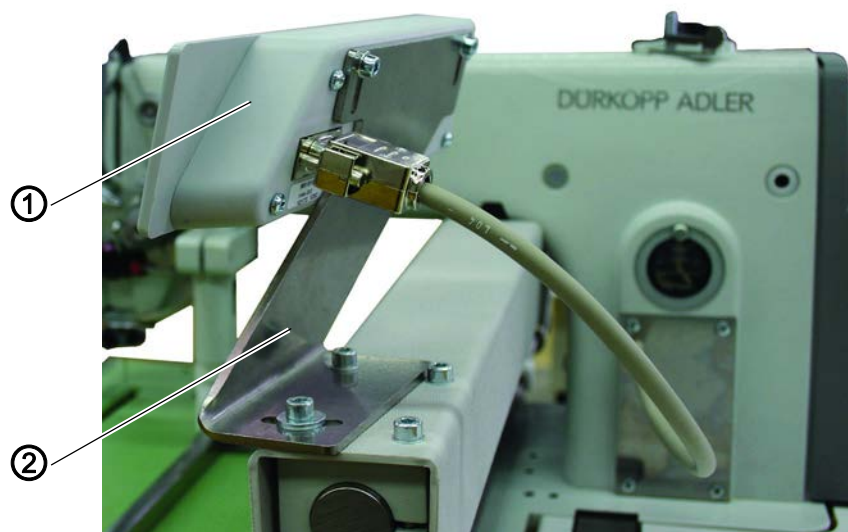
Fig. 34: Assembling the operating panel OP3000
