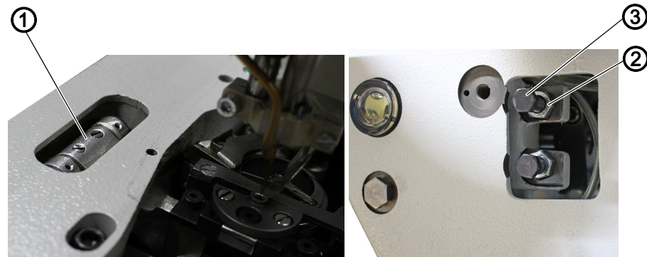
Fig. 4: Setting the zero position of the stitch regulator
