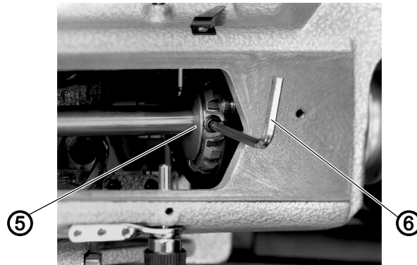
Fig. 44: Setting the position of the integrated adjusting disk relative to the arm shaft (2)
