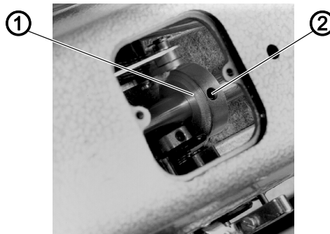
Fig. 54: Resetting the winder wheel
